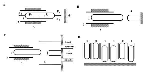
**Fig. 2** Schematics of memory cells based on DWNTs (in position 'on'). 1 is the movable inner wall; 2 is the fixed outer wall; 3, 4 and 5 are the first, second and the control electrodes. A) a memory cell with a flat second electrode; B) an 'all-carbon' memory cell with a carbon nanotube attached to the second electrode; C) an 'all-carbon' memory cell with a control electrode made of a nanotube. D) shows an example of the storage produced from memory cells.
