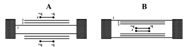
**Fig. 4** Schematics of a nanoactuator: A) a nanoactuator with the inner wall 1 as a stator, B) a nanoactuator with the outer wall 1 as a stator. The walls 1 and 2 comprise the rotational nanobearing, the walls 3 and 4 are the bolt-nut pair with the thread-like shape of the interval interaction energy.
