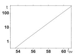
Fig. 3 Dependence of the lifetime (in years) of the 'all-carbon' nanorelay in position 'on' on the overlap of the walls (in nm). The nanorelay contains the (5,5)@(10,10) DWNT as the first electrode and the (5,5) nanotube as the second electrode.
