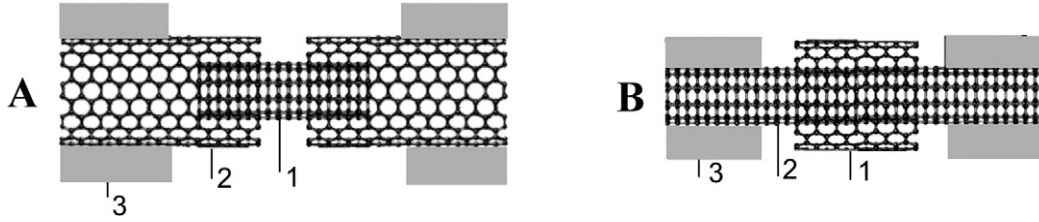
Fig. 3. Schematic of an electromechanical nanothermometer. A: the telescopic nanothermometer with the movable inner wall, B: the shuttle nanothermometer with the movable outer wall. The movable wall is indicated as (1), the fixed wall as (2) and the attached electrodes as (3).
